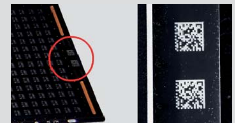
Object: Circuit board with Data Matrix. Image showing high contrast Data Matrix.
