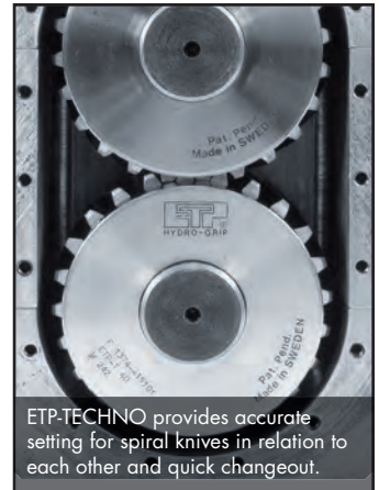
High speeds and frequent mounting in this machine for measuring torque is aided by ETP-TECHNO.
