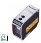
BOD 63M 200...2000 mm 1800 mm BOD000U BOD 63M-LA02-S115 15...30 V DC 0...10 V ≤ 75 mA Light switching
