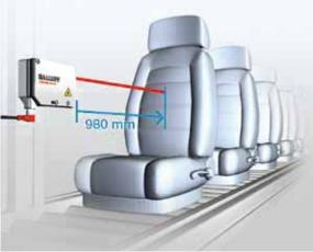
With **distance sensors**, the position-giving target can be any object.
