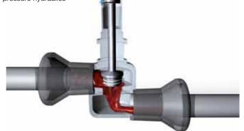
Large valve with controlled actuating drive
