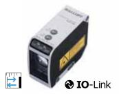
BOD 63M 200...6000 mm 5800 mm BOD0012 BOD 63M-LI06-S4 18...30 V DC 90 mA Light switching 2 yes/yes Teach-in Laser, red light 660 nm 2 per EN 60825 5 mm at 3 m, 10 mm at 6 m 1 mm ≤ 1.5% ≤ ±4 mm ≤ 1.5 mm/K  $\leq \pm 1$  % of Wh ≤ 15 mm ≤ 3.3 ms ≤ 20 ms 150 Hz Green LED Yellow LED Red LED IP 67 -10...+60 °C  $\leq 10 \text{ klx}$ Anodized aluminum Glass
