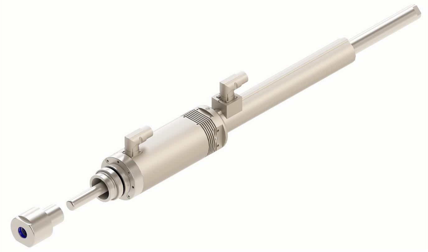
Picture: Front part of the flange, includes sealing and bearings, can be replaced easily. Normally the complete front part with all seals and bearings will be replaced. In case that the seals and bearings are only cleaned the following lubricant has to be used: "fin food Grease 2" from INTERFLON
