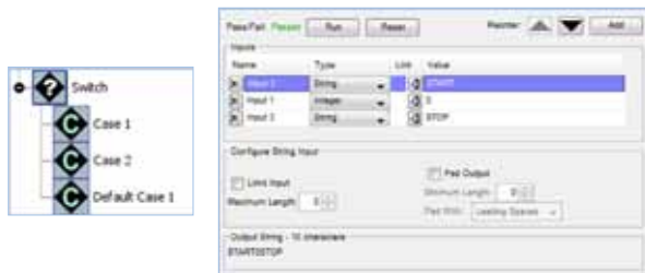
New Switch and String Builder tools to simplify logics and output data formatting
