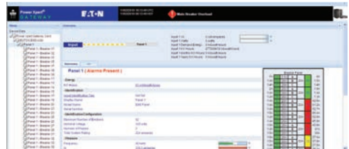
Power Xpert Gateway PDP card—panel view
