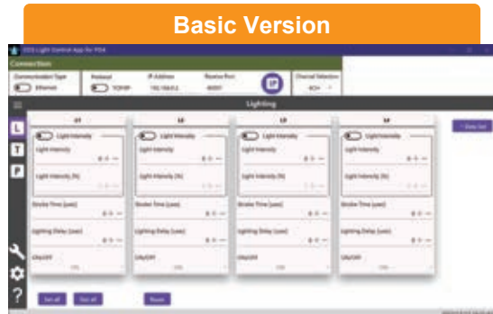
Basic lighting settings such as intensity value and light emission time, as well as trigger input / output settings.
