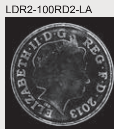
Illuminating from a low angle allows for imaging that emphasizes the edges.
