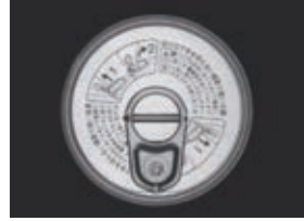
With illumination from LWD 85 mm, the bumps of the pull tab alone can be emphasized in the image.
