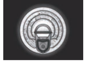
With illumination from LWD 295 mm, all of the bumps on the workpiece surface can be emphasized in the image.
