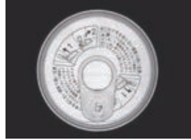
With illumination from LWD 10 mm, the whole surface of the workpiece can be illuminated evenly and the bumps are erased from the image.
