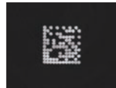
It is possible to determine the 2-D code by evenly illuminating the surface.
