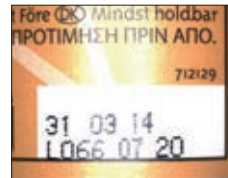
Converged light in the center interferes with stable inspection.
