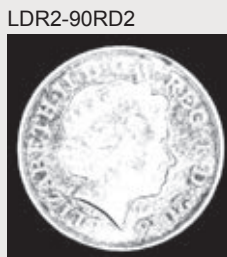
Edge extraction is difficult with illumination from a high angle.
