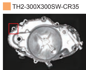
The state of FIPG sealing material can be imaged. The above sample workpiece has been made specifically for sample imaging and is not the one for actual inspection.
