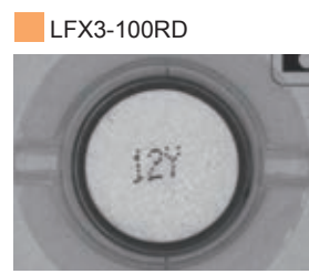
Effects from the textured surface are suppressed so that the characters stand out clearly.
