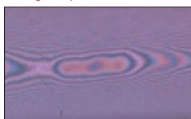
Visualized lamination anomaly with light for interference fringe inspection
