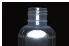
It is difficult to form an image of the liquid level due to surface reflection.
