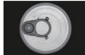
The printed ink transmits infrared light so that the texture of the top surface is evenly captured.
