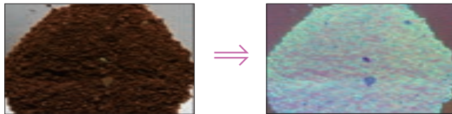
Imaging of foreign matters in coffee powder at 400 nm to 900 nm
