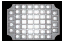
Converged light in the center interferes with stable inspection.
