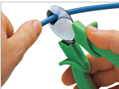
Cutting of cable
