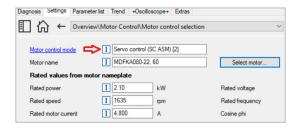
The 24V HTL encoder must also be configured in this case. Wire to DI3 and DI4, set "Input function (P410:002)" to "High resolution HTL encoder [1]," and enter the encoder's number of pulses per revolution (PPR) into "Increments/revolution (P341:001)."
