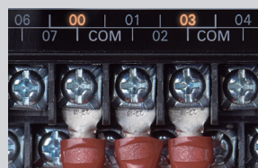
Input/output terminal LED indicators for quick troubleshooting
