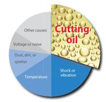
~30% of component failures are caused by cutting oil ingress
