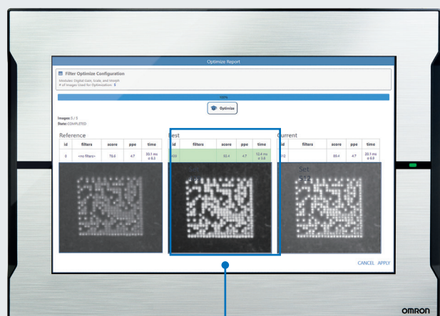
Output – Best filter and parameter set that creates clearest image of the barcode
