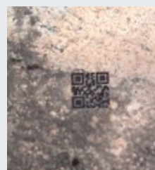
Aluminum casting, no base treatment Cell size: 0.127mm
