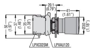
Flush pushbutton with test element and spring-clamp terminal contact or LED elements LPXCS... - LPXLPS...
