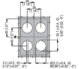
① When Faston contacts are used, the vertical pitch must be 85mm minimum.
