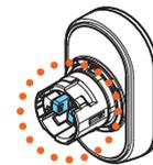
The middle contact activation, with respect to the right and left side contact, can be changed by the user, if required, by removing one mechanism pin. Consult the relative instructions available online in the Downloads section at [www.LovatoElectric.com](http://www.LovatoElectric.com).
