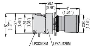
Flush pushbutton with test element and spring-clamp terminal contact or LED elements LPXCS... - LPXLPS...
