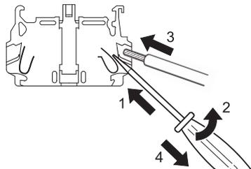
Cable removal (always using flat-blade screwdriver)
