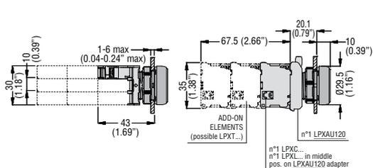
Flush pushbutton with Faston contact elements
