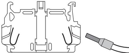
Wiring with flat-blade screwdriver (for flexible bare cable without terminal)
