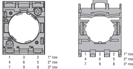
Mounting adapters with contact elements
