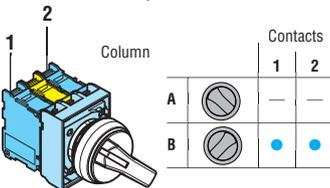
Contact activation of 3-position selector switch
