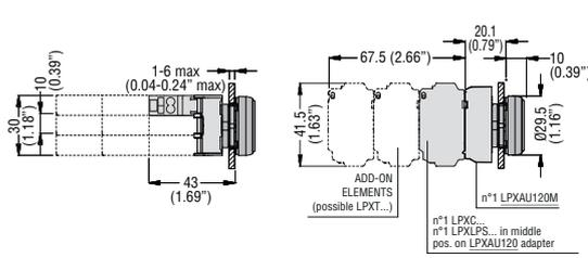
Drillings - Minimum recommended distances with spring-clamp terminal contact or LED elements
