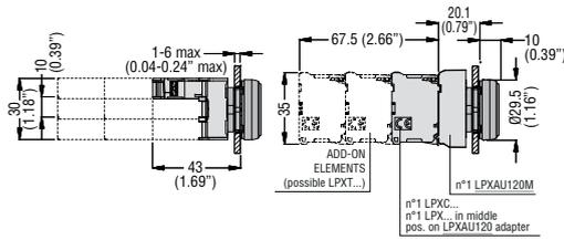
Flush pushbutton with Faston contact elements
