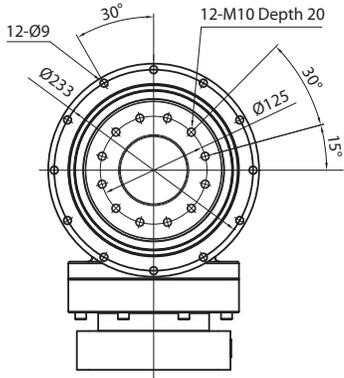
Input bore size  $\leq \text{Ø}38\text{mm}$
