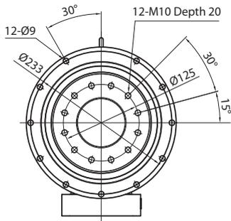
Input bore size  $\leq \varnothing 28\text{mm}$
