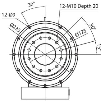
Input bore size  $\leq \varnothing 38\text{mm}$
