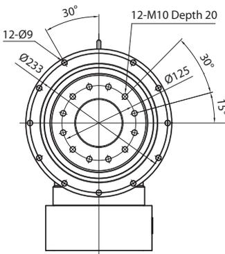
Input bore size  $\leq \varnothing 48\text{mm}$
