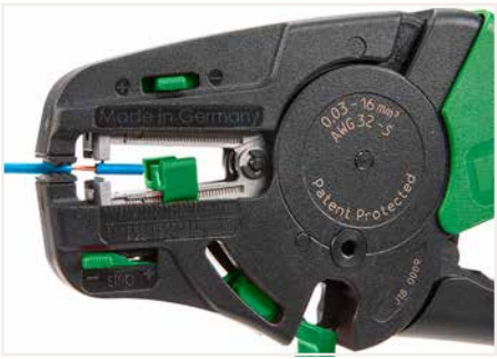
Partially stripping a conductor.
