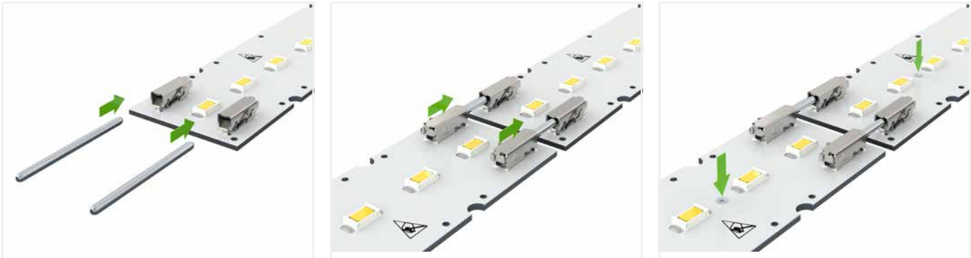
Inserting board-to-board links into the terminal blocks.
