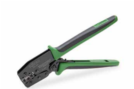
Crimping tool 25; for insulated and uninsulated ferrules; crimping range: 10 mm² (8 AWG), 16 mm² (6 AWG) and 25 mm² (4 AWG)
