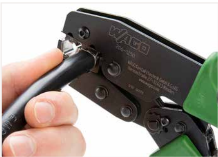
Squeeze handles until ratchet mechanism is released.
