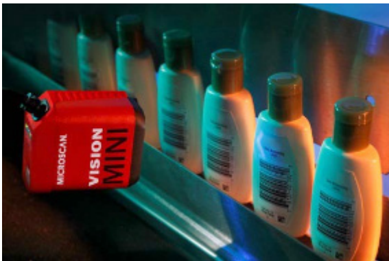
Figure 9: Microscan Vision MINI Smart Camera used for label inspection
